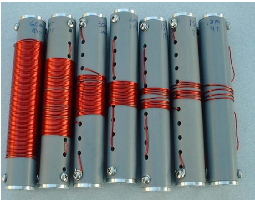
A complete set of coils for 60, 40, 30, 20, 17, 15, and 12M. For 10M you can use the 15 or 12M coil with the whip collapsed for tuning or use a short jumper across any of the lower frequency coils.
